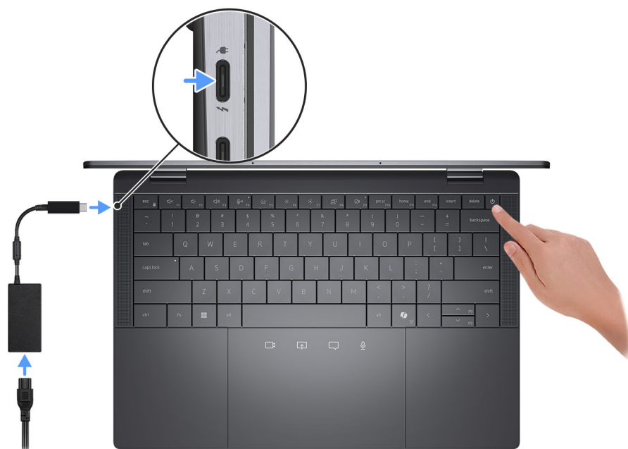
Figure 11. Connecting the power adapter
