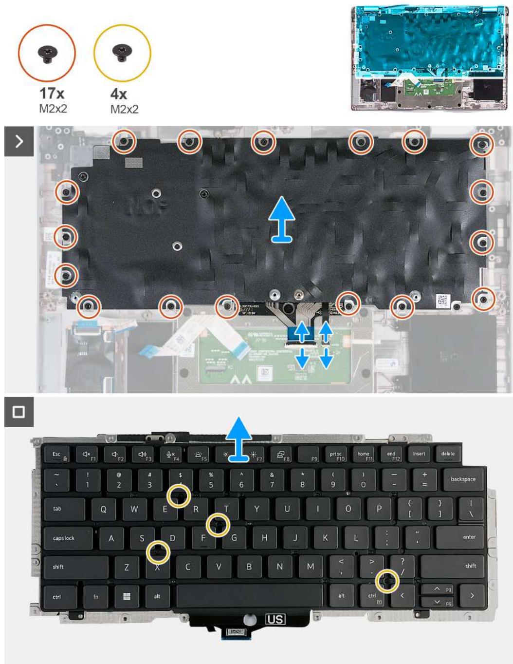
Figure 61. Removing the keyboard
