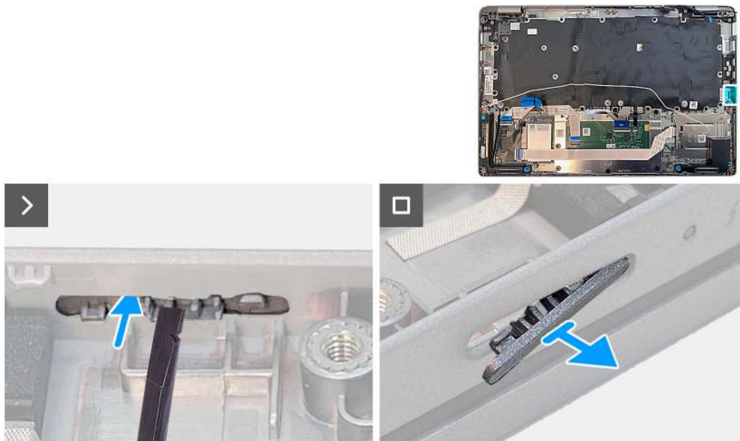
Figure 65. Removing the dummy SIM-card slot filler
