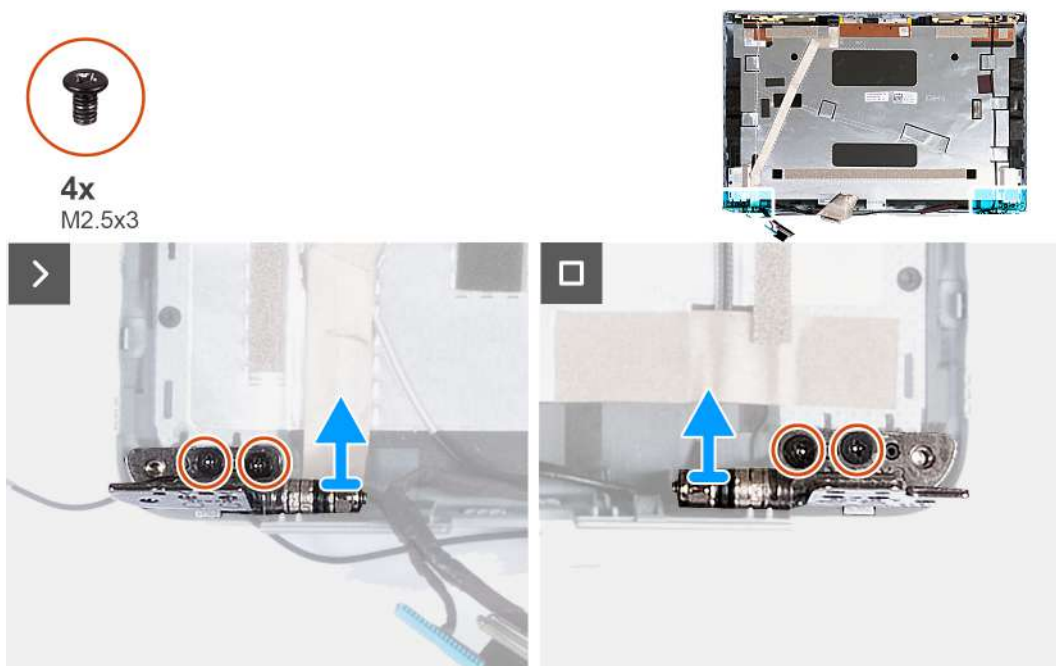
Figure 47. Removing the display hinges
