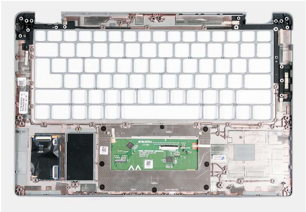
Figure 63. Removing the palm-rest assembly
