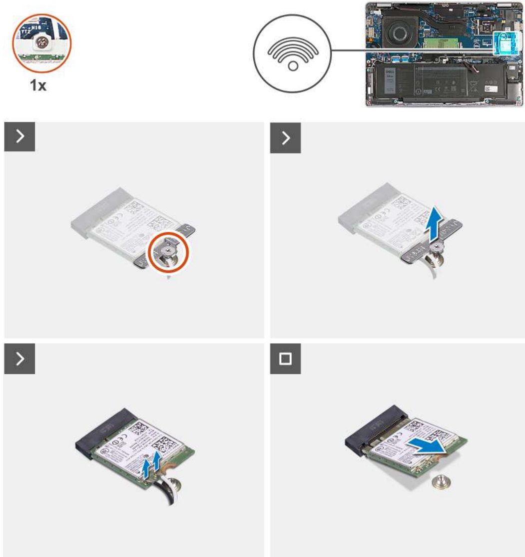
Figure 10. Removing the wireless card
