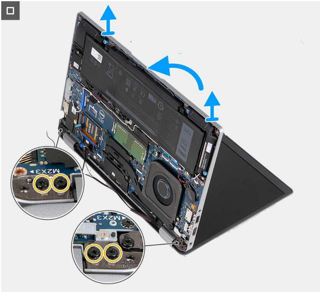
Figure 34. Removing the display assembly - For computers shipped with 4G card
