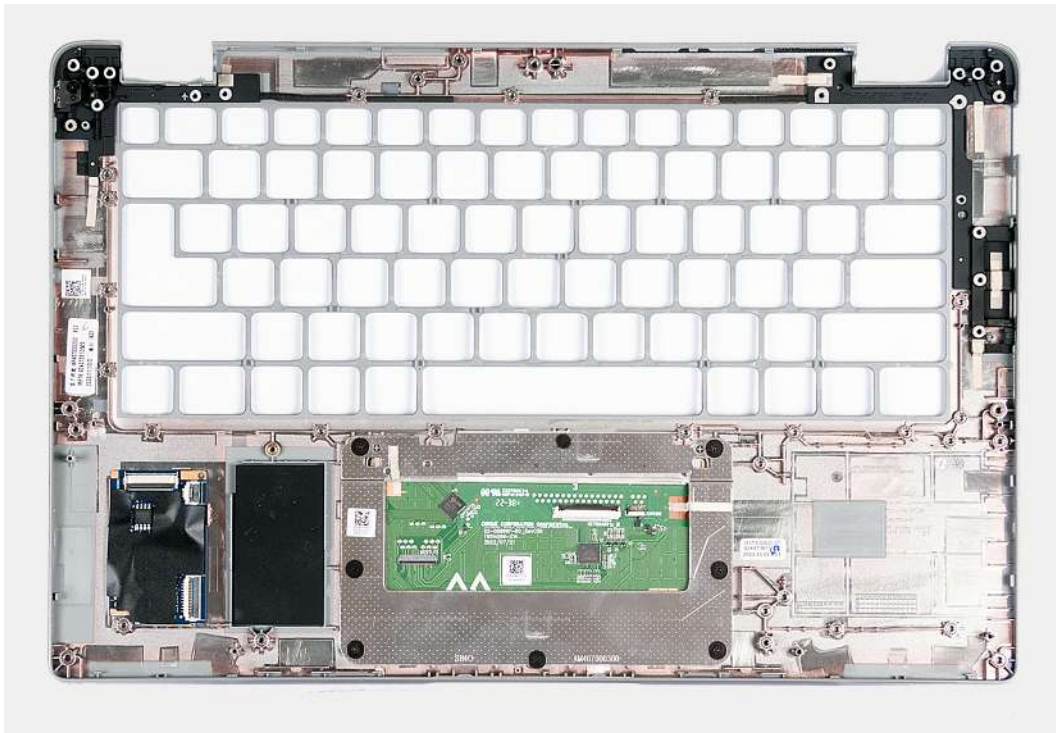
Figure 64. Installing the palm-rest assembly
