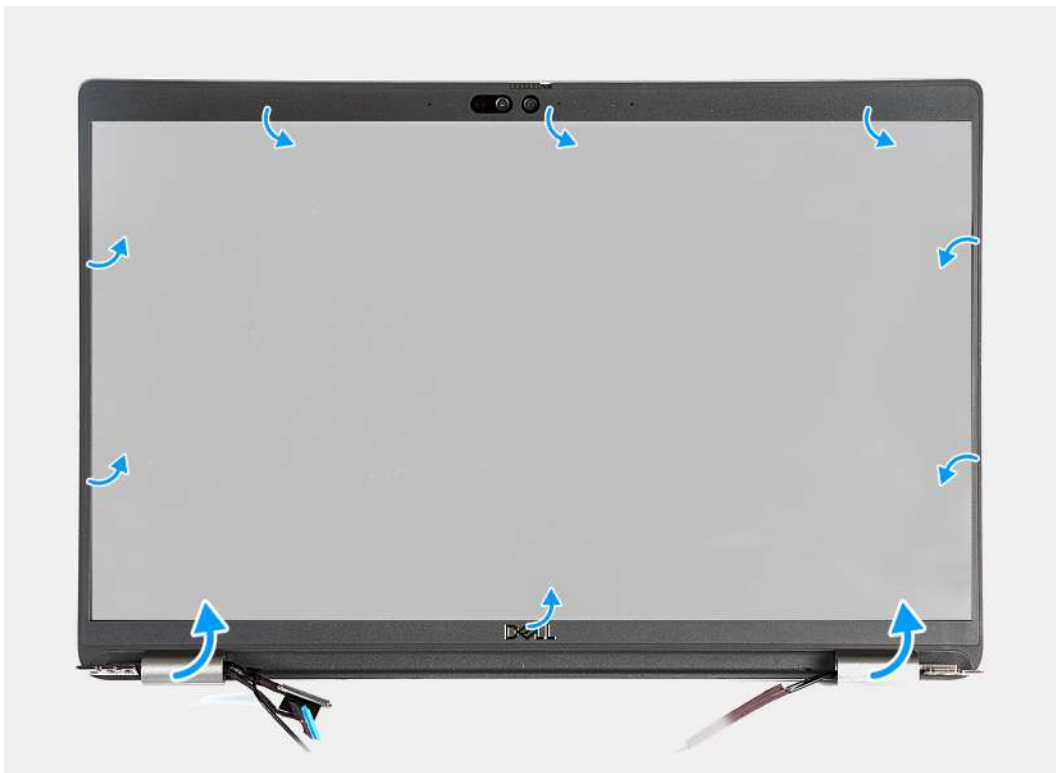
Figure 41. Removing the display bezel
