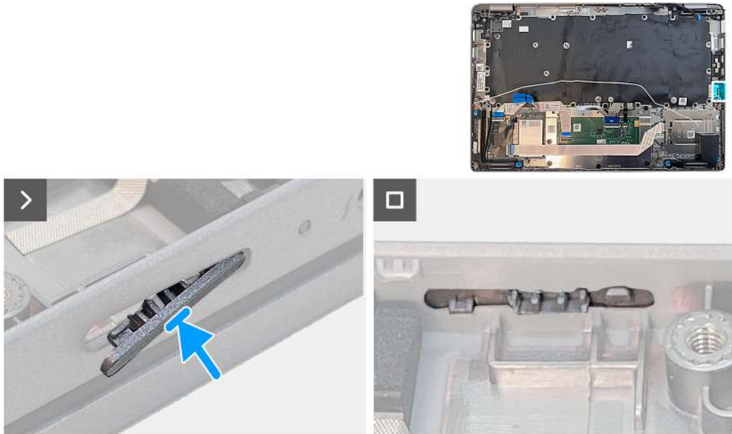
Figure 66. Installing the dummy SIM-card slot filler
