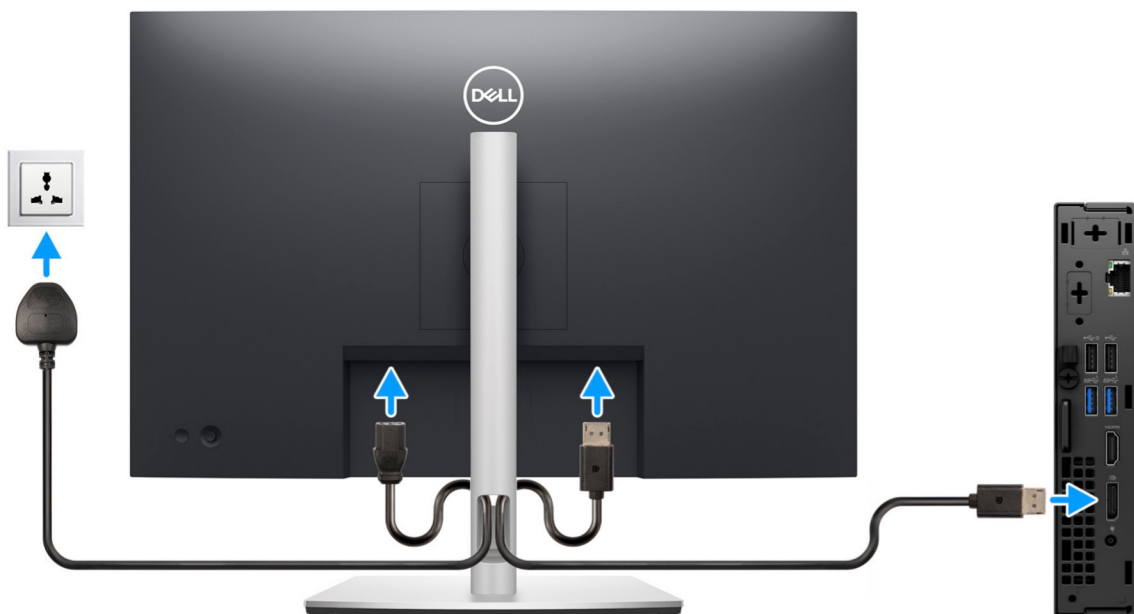
Figure 5. Connect the display
